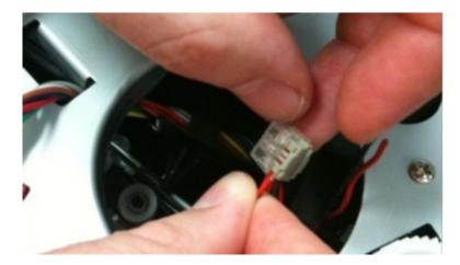
**f** Insert the red wire from the clutch into the IDC.
