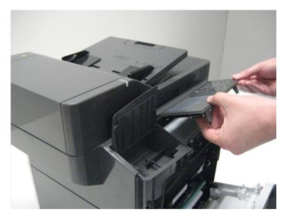
**5** Disconnect the cave LED cable from the controller card.
