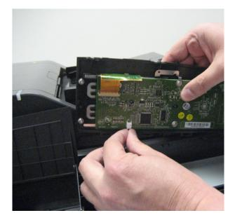
6 Remove the screw (B) to release the toroid holder, and then slide the toroid holder away from the UICC connector.
