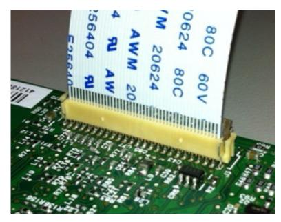
**3** Rotate the locking actuator to the locked position by pressing down on both ends of the actuator. The cable should not move when this step is performed. If the cable moves, open the actuator, reposition the cable, and then close the actuator to the down position.
