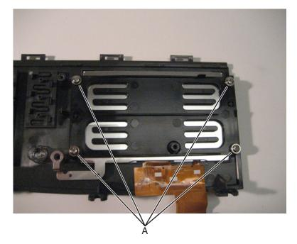
**4** Remove the ground shield.
