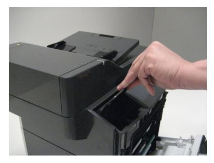
**4** Lift the control panel to access the UICC underneath.
